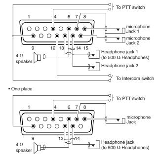
Either intercom or yoke-mounted channel/frequency exchange switch can only be installed. Both switches cannot be installed at the same time.
